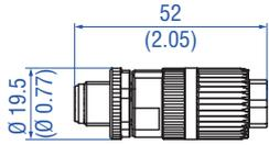
**M12 D-coded male connector (4 pin), straight**
