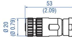
**M12 A-coded female connector (4 pin/5 pin), straight**
