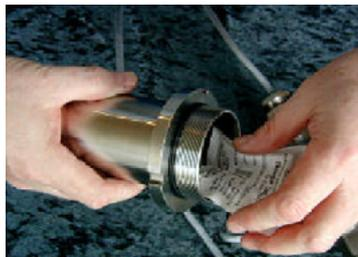
**4.6** Assemble the top and bottom turning clockwise and tighten firmly until top and bottom flanges come together. (see fig. 11) Tighten the cable glands according to manufacturer's specifications.
