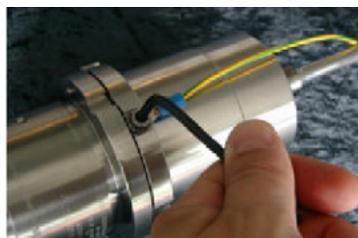
**6.** Tighten the lock screw with min. 1.5 Nm torque.
