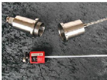
2. Remove rod or profile from the sensor. Separate the plastic tube from the sensor.
