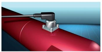
③ Four standard screws must be tightened to mount the connector system on the cylinder. In case of using angled type connectors the connector insert can be rotated inside the flange in 45° steps.
