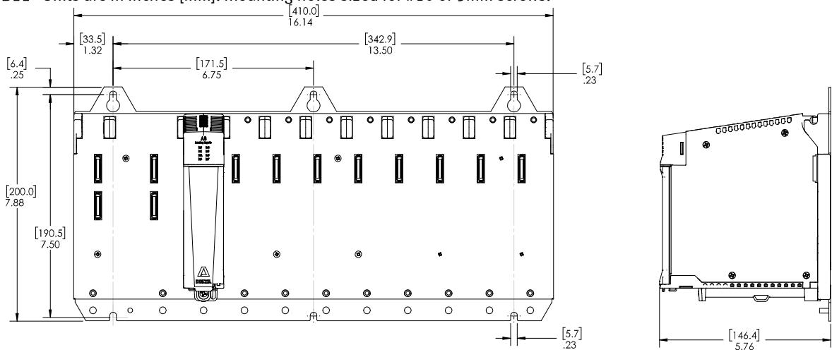
**B15** Units are in inches [mm]. Mounting holes sized for #10 or 5mm screws. The PS6D heat sink protrudes beyond the left of the base by 0.20 inches.
