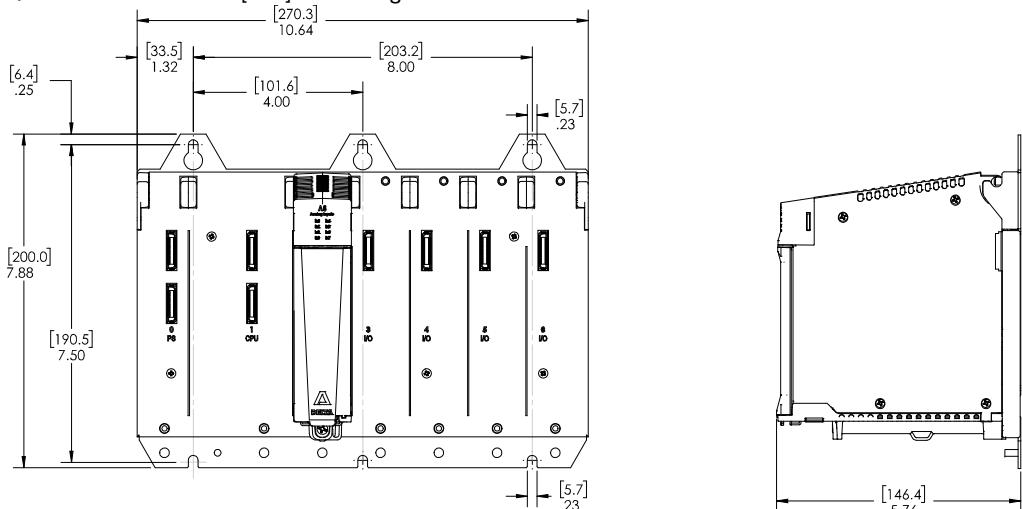
**B11** Units are in inches [mm]. Mounting holes sized for #10 or 5mm screws.
