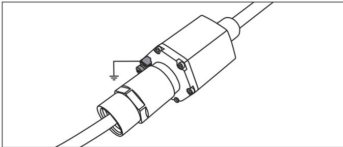
Fig. 20: Grounding via ground lug (version E)
