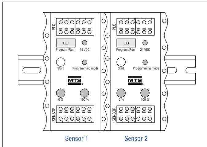
Fig. 28: Dimensions: 10 × 55 × 31 mm (0.39 × 2.17 × 1.22 in.); material: Aluminum, side caps PA 6.6 FR; connection type: Spring terminals, max. 1.5 mm<sup>2</sup>; ingress protection: IP20
