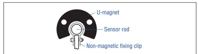
Fig. 16: Example of sensor support (part no. 561 481)
