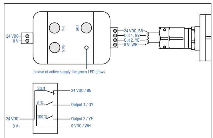
Fig. 24: Connect hand programmer (see connection wiring Fig. 21)
