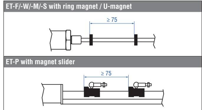
Fig. 18: Examples: Minimum distance for multi-position measurement
