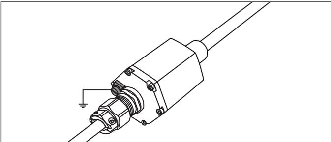
Fig. 19: Grounding via ground lug (version A, N)
