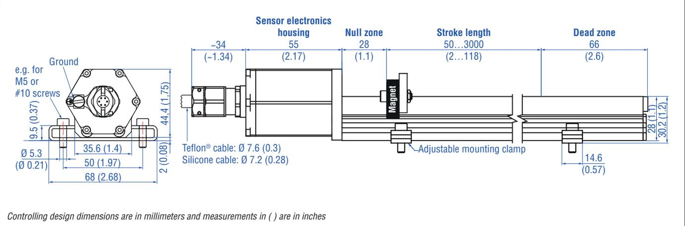
Fig. 9: Temposonics® ET (profile sensor) with U-magnet
