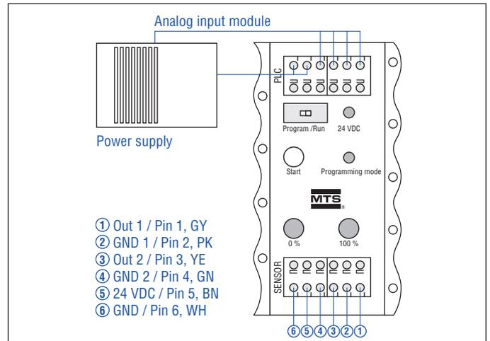
Fig. 29: Connect cabinet programmer (see connector wiring Fig. 21)
