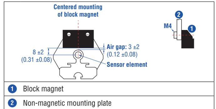
Fig. 14: Mounting of block magnet (part no. 403 448)
