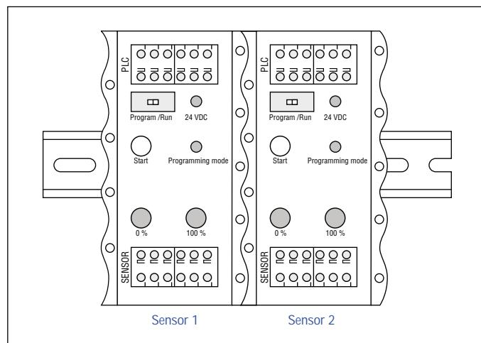
Fig. 36: Dimensions: 10 × 55 × 31 mm (0.39 × 2.17 × 1.22 in.); material: Aluminum, side caps PA 6.6 FR; connection type: Spring terminals, max. 1,5 mm<sup>2</sup>; ingress protection: IP20
