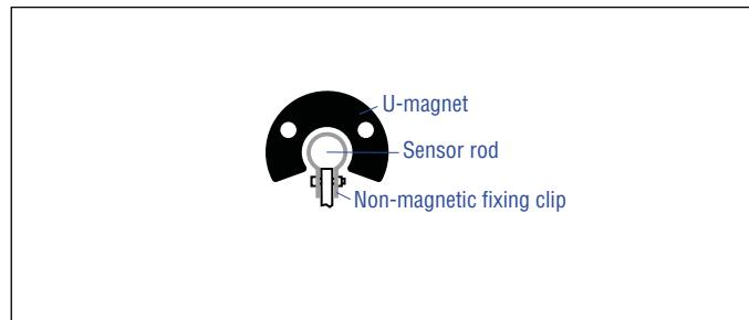
Fig. 19: Example of sensor support (part no. 561 481)
