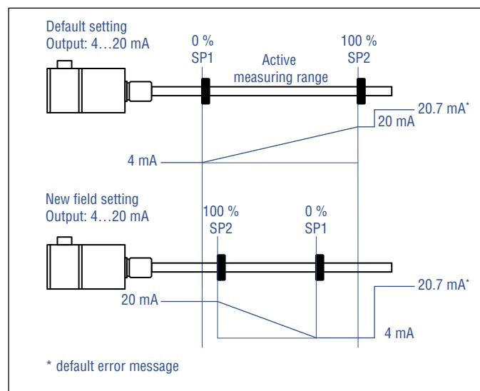
Fig. 46: Start- and endpoint, set the direction
