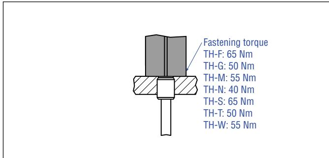
Fig. 11: Mounting example of threaded flange
