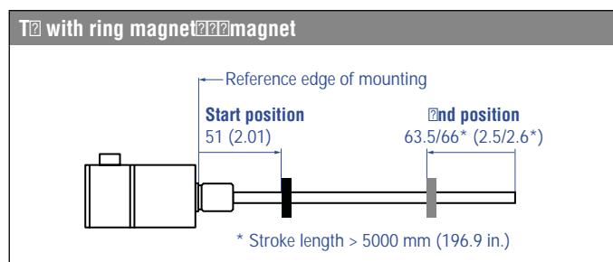
Fig. 20: Start and end positions of magnets
