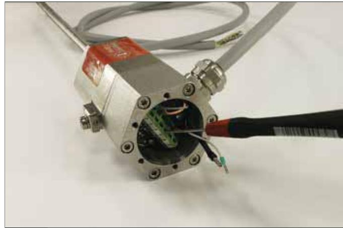
3 Connect the cable to the sensor.
