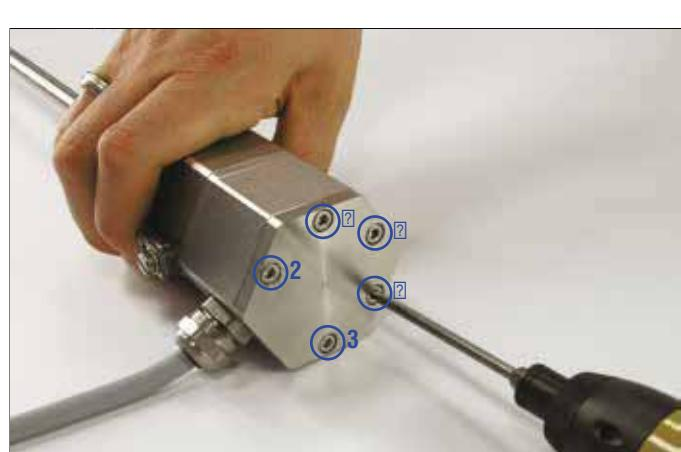
4 Inspect surfaces and O-ring for damage. Wipe surfaces clean and apply O-ring lube. Check the position of O-ring between upper lid and connection adapter.
