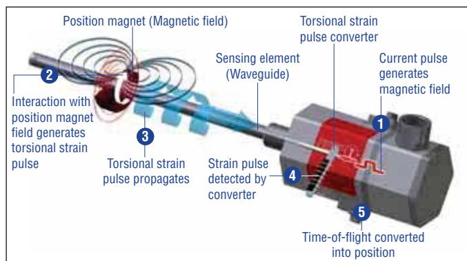
Fig. 4: Time-of-flight based magnetostrictive position sensing principle
