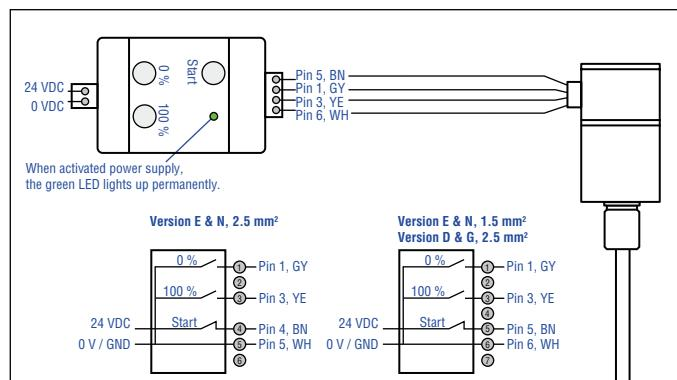
Fig. 32: Connect hand programmer (see connection wiring Fig. 26/Fig. 27/Fig. 28 on page 20)
