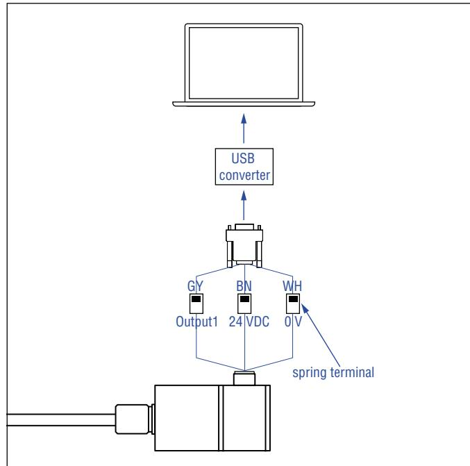
Fig. 40: Connect PC programmer (with spring terminal)
