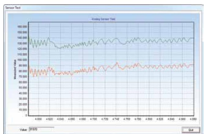
Fig. 44: Sensor Test diagram of analog sensor with 2 position magnets
